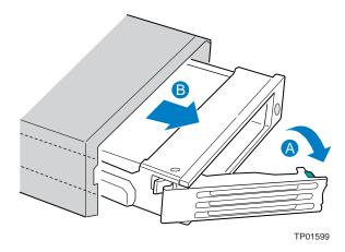
Figure 16. Removing a Hot-swap Hard Drive Carrier from Chassis
